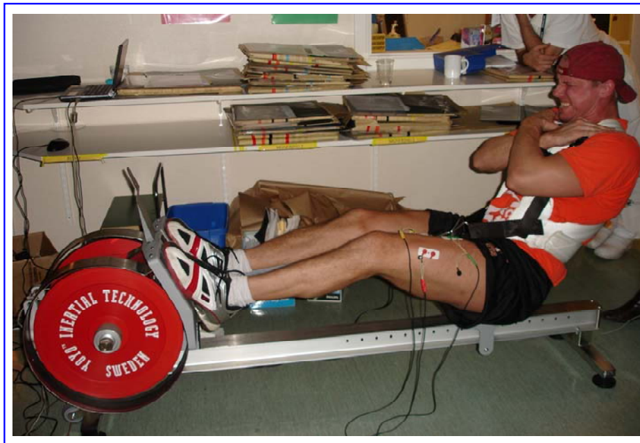
Figure 1. Subject performing the equivalent of squat exercises on the Flywheel Multigym. The subject is wearing an harness connected to the flywheel axle, which is put into rotation (CON action) when he is pushing with his legs against the foot rests, thus sliding backwards on the rails. The subsequent coupled ECC action consists of resisting to the pulling force of the flywheel after the strap has been unwound and starts to recoil.
