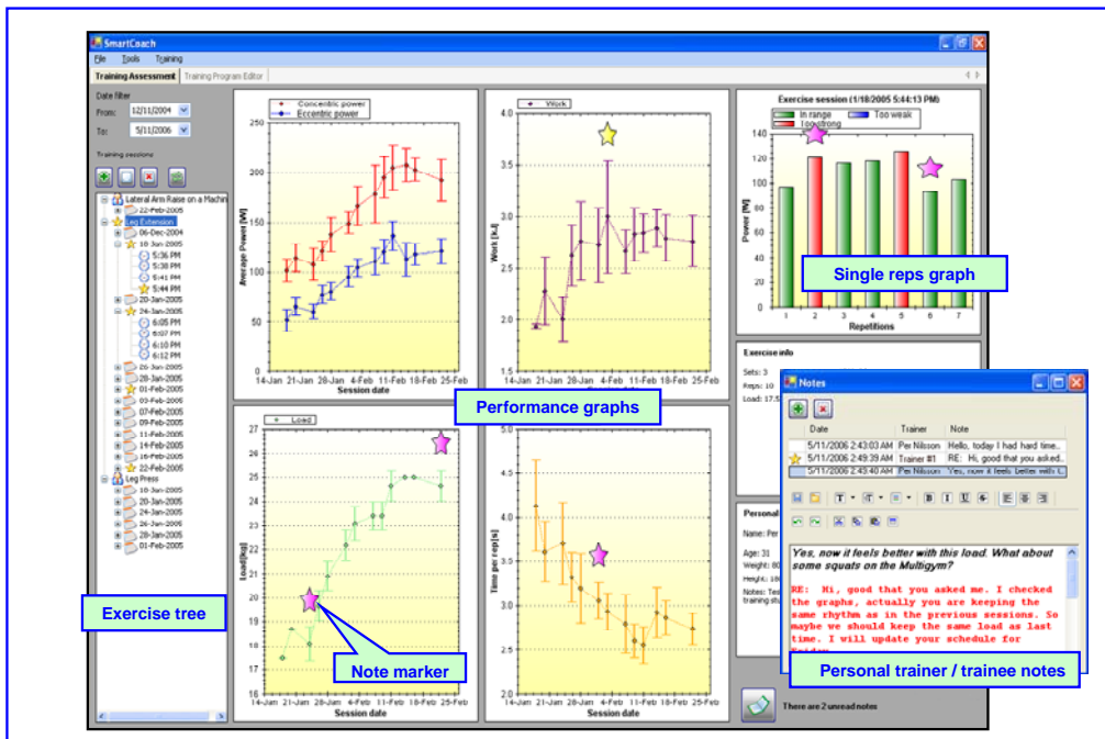
Figure 3. The performance assessment window. All the exercises performed can be browsed from the exercise tree; the evolution of performance parameters during training can be viewed in the performance graphs, as well as during single exercises (single reps graphs). The remote trainer has full access to the trainee's data set by means of the remote connectivity feature. Both the trainee and his remote personal trainer can post general or specific notes (note marker). Such system is also used by the trainer to give guidelines to the trainee or edit his training schedule (Figure 4) if needed.
