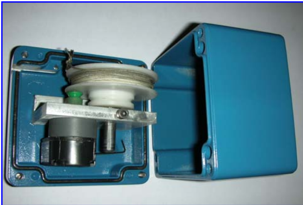
Figure 2. Left: the mechanical part of the encoder for power measurement. It has a robust construction and features easily maintenance (e.g., in case of substitution of the wire). Right: the instant power feedback window, which guides the trainee during the execution of his exercise with a given target power.
